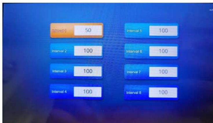
(2) Current sensitivity interval display: There are 8 intervals from 1 to 8, each allowing separate sensitivity settings. Click on the interval to modify and input the corresponding sensitivity (Interval 1 defaults to 50, others default to 100). Click "Close" to exit the interface and return to the main interface by clicking the upper left corner.
