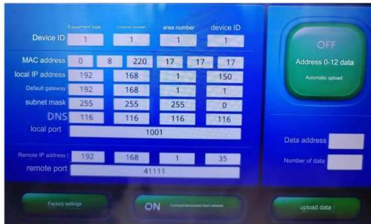
Current display network configuration interface: Click the "other Settings" icon to enter the network configuration options. The security gate has networking functions. Once the configuration connection is completed, the data can be synchronized to the background computer for viewing and parameter modification. Additionally, you can set up email reminders; when abnormal alarm values are detected, notifications can be sent to the specified mailbox.
