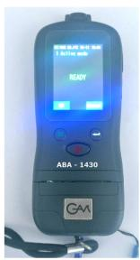
**GANM™ ABA – 1430 (BIP)** is a hand held, portable breath alcohol tester to check subject's breath Alcohol concentration with reliable accuracy. It has a built-in printer to provide evidential receipts showing driver's name, address, Driving license no., Vehicle Number, police id, alcohol content, date & time of test etc.
