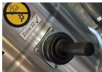
Scuotifiltro manuale laterale Side-mounted manual filter shaker
