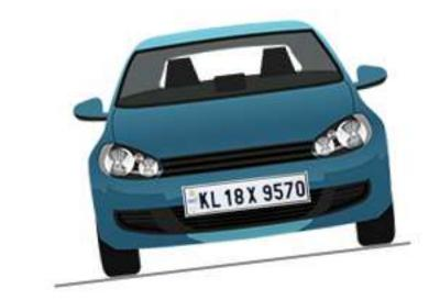
The angle of the number plate should not exceed 5 degrees (clock or anti clockwise).
