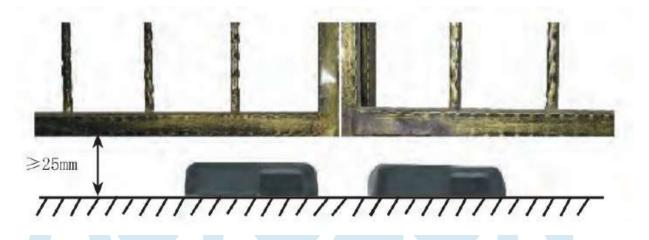
2. The unevenness of the ground within the working scope of the gate opener. Fall h=Height of the highest point of the ground- height of the lowest point of the ground.
