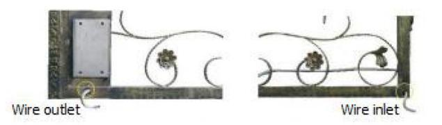
4. Fix the gate opener and connect the wires (whose color shall be the same as label of terminal block of the control box or the color of the plug wire).
