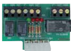
ACQ9081 3 Relay Card for P1 to manage courtesy light, traffic light, electromagnetic lock with P1-CRX
