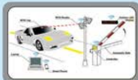
Automatic Parking Management system
