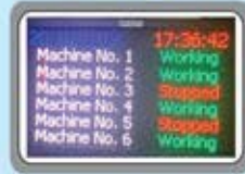
Operational LED Display Board
